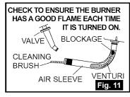
inch to prevent pushing any debris further into the tube. (see Figure 11)
